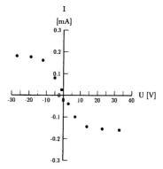
Fig. 1. Double probe characteristics at the pressure of 60 Pa. Plasma parameters calculated from this curve are as follows: Electron temperature 4.5 eV, plasma density  $1.5 \times 10^{16} \text{ m}^{-3}$ , Debye length  $1.3 \times 10^{-4} \text{ m}$ .
