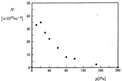
Fig. 2. Oxygen plasma density vs. pressure in the discharge vessel.
