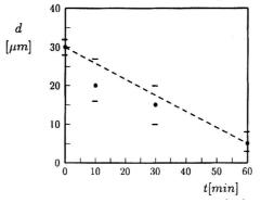
Fig. 3. Polymer foil thickness vs. duration of plasma treatment.
