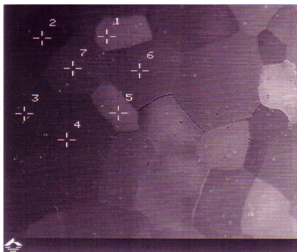
Fig. 1. Scanning electron microscopy image of corresponding points on different grains of measured AES spectra of antimony surface segregation.
