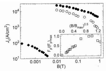
Fig. 6. Plot of the critical current density vs. field B, at T=81 K, for the ceramic Bi 2223 sample  $S_A$  ( $\diamond$ ) and Bi 2223 tape ( $\bullet$  and  $\circ$  for B parallel and perpendicular to the plane of the tape, respectively). The inset: plot of volume pinning force  $F_p=J_cB$ , normalized to its maximum value vs. normalized field showing a  $F_p\sim B^{0.5}$  variation in Bi 2223 tape.
