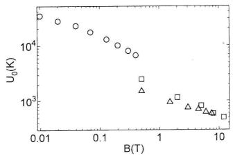
Fig. 4. Pinning potentials  $U_0$  for the core of Bi 2223 tape ( $\circ$ ), epitaxial Bi 2223 film ( $\square$ , Ref. [6]) and Bi 2223 whisker ( $\triangle$ , Ref. [12]) versus field (parallel to the crystalline c-axis).
