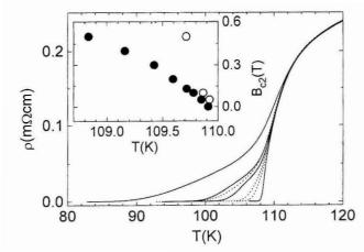
Fig. 2. Resistive transitions for the core of Ag-Bi 2223 tape in field:  $B=0,\ 0.05,\ 0.1$  and 0.5 T (right to left) applied parallel (- - - - ) and perpendicular (——) to the plane of the tape. The inset: the plot of upper critical fields  $B_{C2}^c(\bullet)$  and  $B_{C2}^{ab}$  ( $\circ$ ) for the same tape versus temperature.
