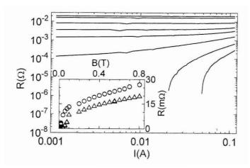
Fig. 5. Plot of resistance vs. current for the bare core of Ag-Bi 2223 tape at T=100 K for fields B (parallel to c-axis) = 0.01, 0.02, 0.04, 0.06, 0.08, 0.1, 0.5 and 0.8 T (bottom to top). The inset: plot of the Ohmic resistance vs. field B for a bare core of the Bi 2223 tape at T=100 K ( $\triangle$ ) and 103 K ( $\bigcirc$ ). Note the flux-flow at higher B.
