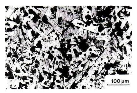
Fig. 2. Optical micrograph of the YBa<sub>2</sub>Cu<sub>3</sub>O<sub>7-x</sub> ceramic, sample NOZ 1-II (aged for 70 hours at 960 °C), polished with diamond paste and etched for 5 seconds in a mild solution of HCl in distilled water.
