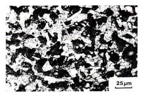
Fig. 1. Optical micrograph of the YBa<sub>2</sub>Cu<sub>3</sub>O<sub>7-x</sub> ceramic, sample NOZ 1-I (aged for 7 hours at 960 °C), polished with diamond paste and etched for 5 seconds in a mild solution of HCl in distilled water.
