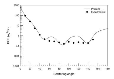
Fig. 5. Differential cross sections for electron scattering from Yb atoms at energy 80 eV.
