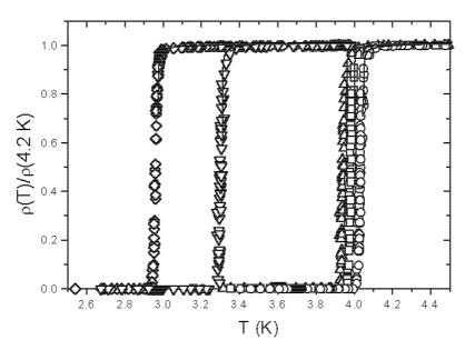
Fig. 3. The temperature-dependent electrical resistivity relative to its value at 4.2 K,  $\rho(T)/\rho(4.2\,\mathrm{K})$ , versus temperature below 4.5 K of  $\mathrm{Zr_{80}Co_{20}}$  metallic glasses: unrelaxed ( $\square$ ), the thermally relaxed up to 563 K with s=60 K/min ( $\bigcirc$ ), the thermally relaxed up to 563 K with s=10 K/min ( $\bigcirc$ ), the thermally relaxed up to 618 K with s=10 K/min ( $\bigcirc$ ), the thermally relaxed up to 653 K with s=60 K/min ( $\bigcirc$ ).
