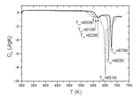
Fig. 1. The temperature dependence of  $C_{\rm p}$  of the  $\rm Zr_{80}Co_{20}$  metallic glass in the temperature range of 298 – 723 K at the heating rates, s: s=60 K/min (full line), s=30 K/min (dashed line), s=10 K/min) (dotted line).
