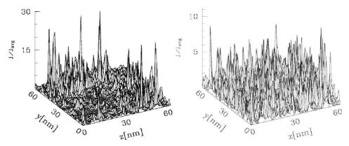
Fig. 3. This figure is related to the same data set as the previous one. It shows the current density distribution at the distance x=55 nm from the injection electrode, as obtained for the ensemble of 64 two-dimensional plates (i.e. 3D correlated energy landscape). The z=35 nm cross-sections of these figures correspond to the cross-sections at x=55 nm of Fig. 2. The homogenization of the charge flow caused by the ordered injection layer is visible by comparing the two figures. F=0.5 MV/cm.
