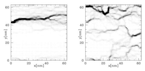
Fig. 4. The current density profiles for electric fields for F=1.0 MV/cm and F=0.1 MV/cm. The current is much more inhomogenous for the higher field. At lower fields, the current density lines are much less straight and the meandering contributes to the homogenization of the current flow.
