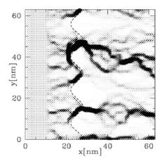
Fig. 5. The effect of a rough organic heterojunction barrier in the interior of the device. The dashed line indicates the heterojunction boundary. The two organic materials are parameterized by the same disorder strength,  $\sigma = 0.07$  eV. The energy barrier at the heterojunction is 0.4 eV. F = 0.5 MV/cm.
