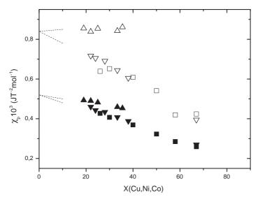
Fig. 2.  $\chi_{\rm p}$  of  ${\rm Zr_{100-}}_x{\rm Co}_x$  ( $\triangle$ ),  ${\rm Zr_{100-}}_x{\rm Ni}_x$  ( $\nabla$ ),  ${\rm Zr_{100-}}_x{\rm Cu}_x$  ( $\square$ ) alloys versus x. The same symbols but full represent dependence of  $\chi_{\rm p}^0$  versus x for the same alloys. Dashed lines extrapolate the data to x=0.
