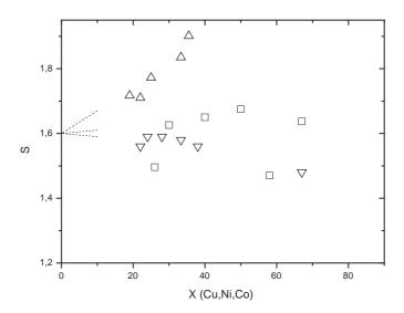
Fig. 3. The Stoner factor of  $\operatorname{Zr}_{100-x}\operatorname{Co}_x(\triangle)$ ,  $\operatorname{Zr}_{100-x}\operatorname{Ni}_x(\bigtriangledown)$ ,  $\operatorname{Zr}_{100-x}\operatorname{Cu}_x(\Box)$  alloys versus x. Dashed lines extrapolate the data to x=0.
