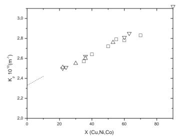
Fig. 4. Modulus of the scattering vector corresponding to the position of the first maximum of the diffraction pattern  $k_p$  of  $\operatorname{Zr}_{100-x}\operatorname{Co}_x(\triangle)$ ,  $\operatorname{Zr}_{100-x}\operatorname{Ni}_x(\nabla)$ ,  $\operatorname{Zr}_{100-x}\operatorname{Cu}_x(\square)$  alloys versus x [22,23]. Dashed line extrapolates the data to x=0.
