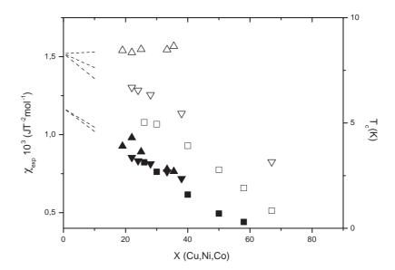
Fig. 1. Measured magnetic susceptibility  $\chi_{\rm exp}$  of amorphous  ${\rm Zr}_{100-x}{\rm Co}_x$  ( $\triangle$ ),  ${\rm Zr}_{100-x}{\rm Ni}_x$  ( $\nabla$ ),  ${\rm Zr}_{100-x}{\rm Cu}_x$  ( $\square$ ) alloys versus x (left scale). The same symbols but full show the variation of superconducting transition temperatures  $T_c$  with x for the same alloys (right scale). Dashed lines extrapolate the data to x=0.
