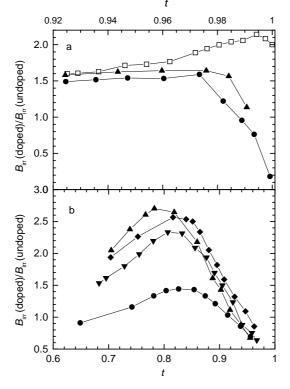
Fig. 3. The ratio  $B_{\rm irr}({\rm doped})/B_{\rm irr}({\rm undoped})$  vs. reduced temperature  $t=T/T_{\rm c0}$  for a) MgB<sub>2</sub> 5 wt% Si-doped wire ( $\square$ ) and tapes with c=5 wt% Si ( $\bullet$ ) and 10 wt% ( $\blacktriangle$ ), and b) Bi2223/Ag tapes with  $B_{\phi}=0.21$  ( $\bullet$ ), 0.37 ( $\blacktriangle$ ), 0.39 ( $\blacktriangledown$ ) and 0.54 T ( $\blacklozenge$ ).
