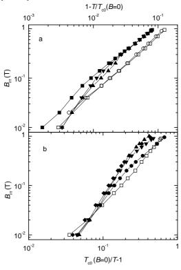
Fig. 2. Temperature dependence of the irreversibility field  $B_{\rm irr}$  in appropriate temperature scales for a) MgB<sub>2</sub> samples: undoped ( $\square$ ) and Si-doped ( $\blacksquare$ ) wire and undoped ( $\bigcirc$ ), 5 wt% ( $\blacktriangle$ ) and 10 wt% Si-doped tape ( $\blacktriangledown$ ), and b) Bi2223/Ag tapes: undoped ( $\square$ ),  $B_{\phi}=0.21$  ( $\bullet$ ), 0.37 ( $\blacktriangle$ ), 0.39 ( $\blacktriangledown$ ) and 0.54 T ( $\bullet$ ).
