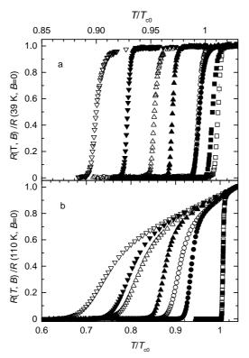
Fig. 1. Temperature variation of the normalized electrical resistance for: a) MgB<sub>2</sub> undoped tape (empty symbols) and tape doped with 5 wt% Si (full) in magnetic fields  $B = 0(\square)$ , 0.1 (O), 0.4 ( $\triangle$ ) and 0.9 T ( $\nabla$ ), b) control Bi2223/Ag tape (empty) and Bi2223/Ag tape with  $B_{\phi} = 0.54$  T (Table 1, full symbols) in  $B = 0(\square)$ , 0.1 (O), 0.4 ( $\triangle$ ) and 0.95 T ( $\nabla$ ).
