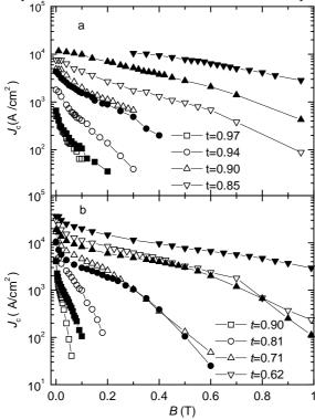
Fig. 4. Field variation of critical current density  $J_c$  at reduced temperatures denoted on plot for the: a) MgB<sub>2</sub> undoped wire (empty) and 10 wt% Sidoped tape (full symbols) and b) Bi2223/Ag undoped tape (empty) and tape with  $B_{\phi} = 0.54$  T (full symbols).
