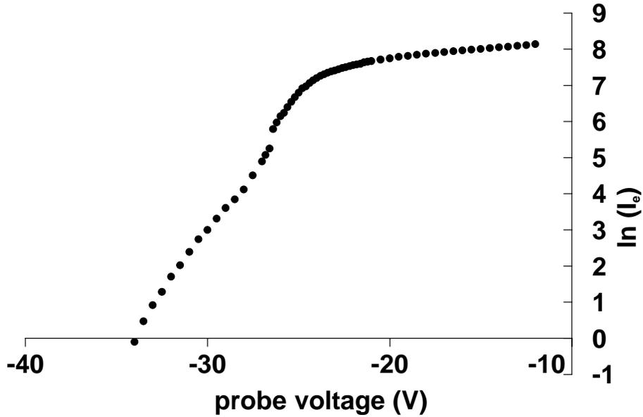
Fig 3. Probe voltage - current characteristic for 100 mA discharge current and 1.33 Pa oxygen gas pressure.
