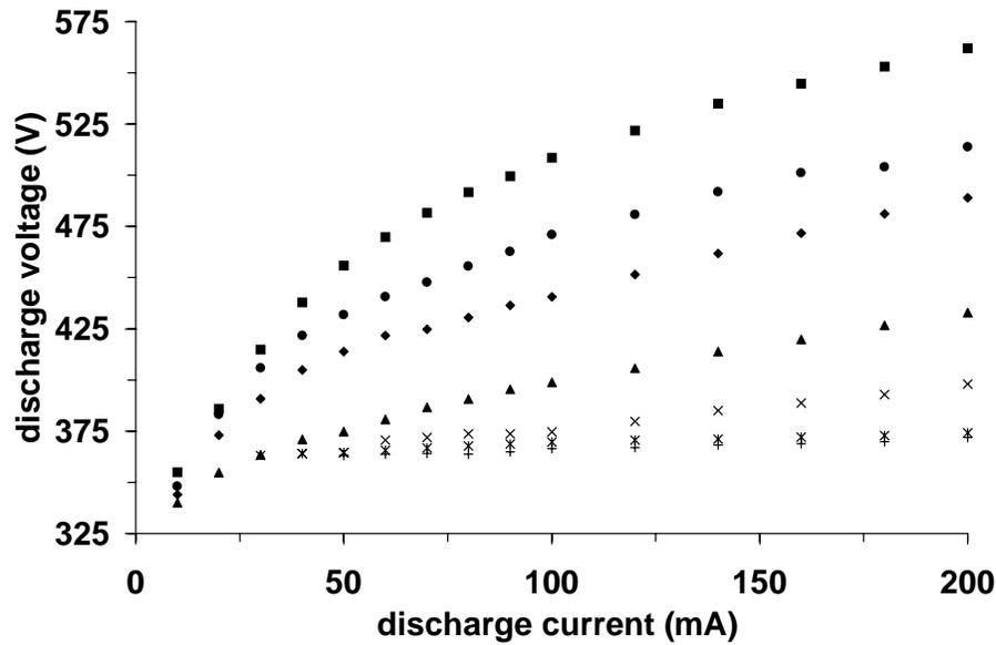
Fig 2. Voltage - current characteristics for seven oxygen gas pressures.
